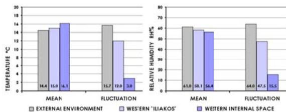
Figure 11a, b: Comparison bars of temperature and relative humidity values of western “iliakos” and internal space.
