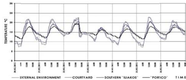
Figure 4: Temperature data of the buildings' outdoor spaces.
